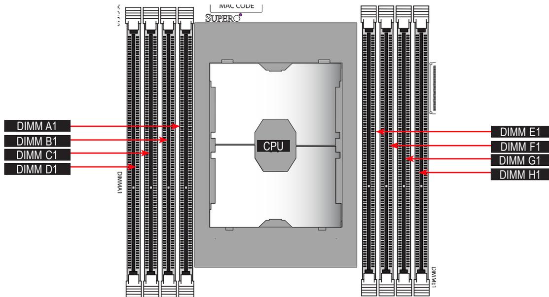
Figure 2-2. DIMM Numbering
