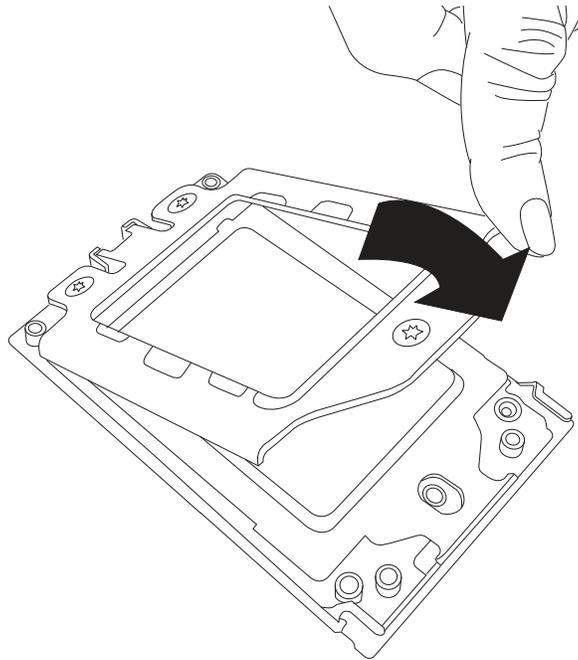
9. Gently lower the force frame down onto the rail frame and hold it in place until it is seated in the Socket housing. Note that the force frame is spring loaded and has to be held in place before it is secured. **Important: Use a torque screwdriver, set it at 16.1 kgf-cm (14.0 lbf-in) with a Torx T20 screw head bit, to prevent damage to the CPU.**
