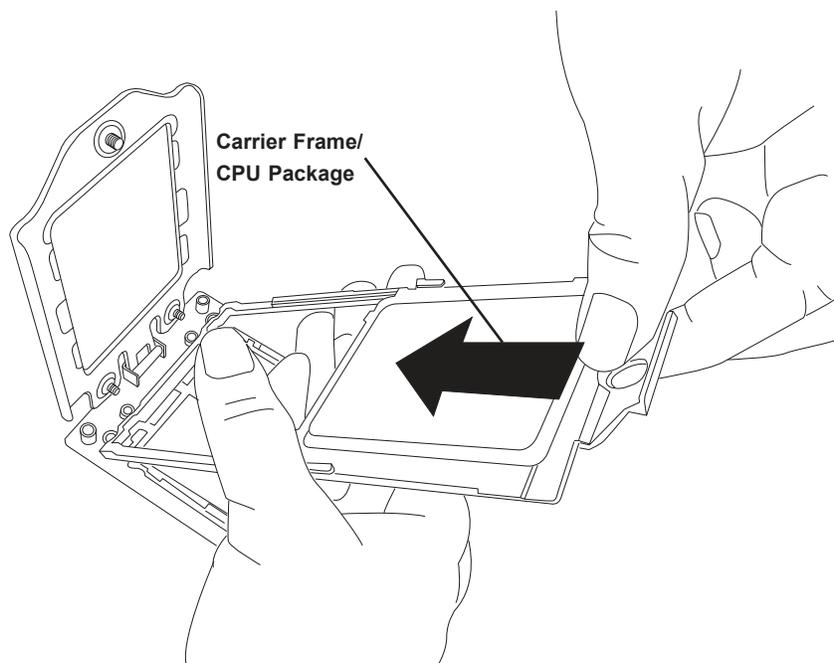
**Note:** You can only install the CPU inside the socket in one direction with the handle at the top. Make sure that it is properly inserted into the CPU socket before closing the rail frame plate. If it doesn't close properly, do not force it as it may damage your CPU. Instead, open the rail frame plate again, and double-check that the CPU is aligned properly.
