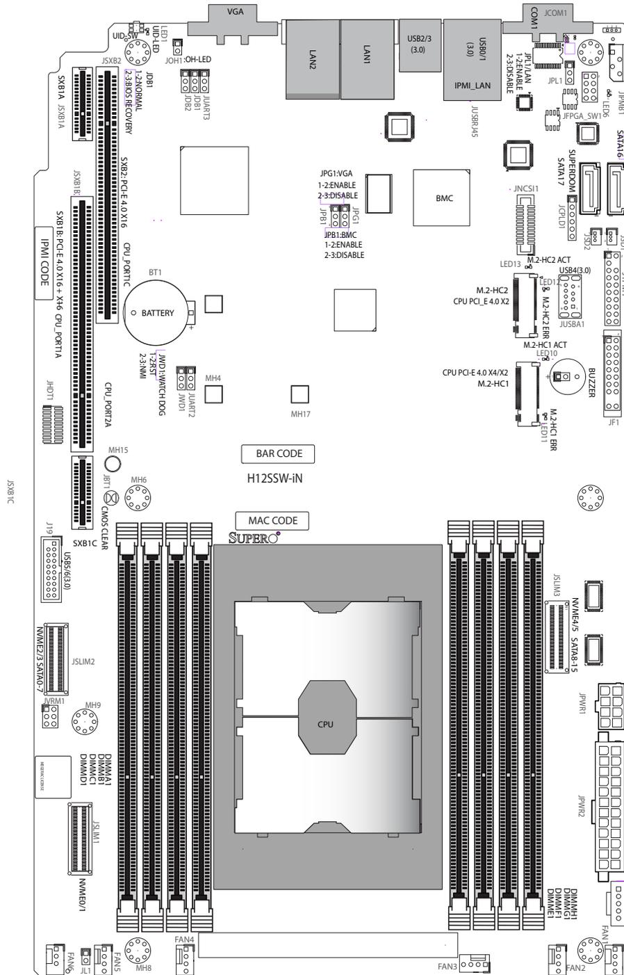
Figure 1-2. H12SSW-iN/NT Layout
