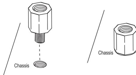
3. Locate the matching mounting holes on the chassis. Align the mounting holes on the motherboard with the mounting holes on the chassis.
